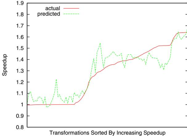
**Figure 1: Model accuracy for *compress*.** The y-axis corresponds to speedup relative to the original untransformed program. The x-axis corresponds to transformation sequences sorted in increasing performance. The line marked *actual* corresponds to the real measured performance and *predicted* corresponds to the model's predictions. The predictions are averaged over 30 trials.
