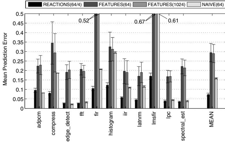
**Figure 5:** Mean prediction error: Reactions, Features and Naive predictors. Averages over 30 trials, 64 training patterns per benchmark, except for FEATURES(1024) which uses 1024 training patterns. 4 canonical transformations were applied for the reaction-based approach.
