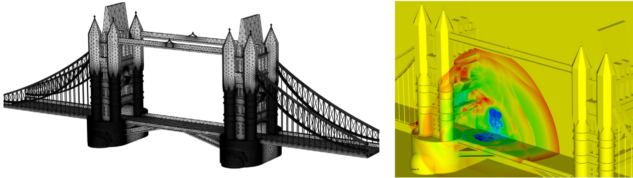
Fig. 11. Tower-bridge test case. Initial mesh and geometry (left) and density iso-values of the blast on an adapted mesh (right).
